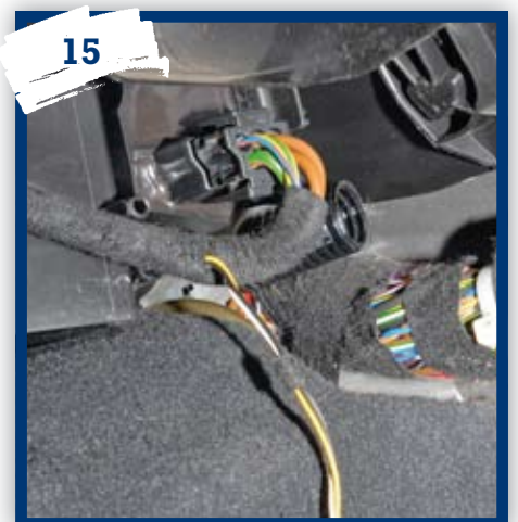
With that lot out of the way, the resistor is revealed.
