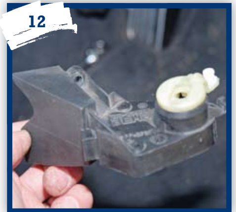
The housing is held by two Torx screws – the lower one you can see, but the upper one is almost impossible to see with your head under the dash, so this shot of the part out of the car shows what you're looking at. You'll need a slim Torx bit to fit inside the moulded gallery for the screw but it will also need to be short enough to clear the steering column. If you're lucky, you can catch it with a small flat-bladed screwdriver but be careful not to round the head off.
