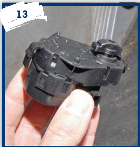
The stepper motor itself is simply unclipped from the housing by squeezing the retaining clips which are moulded into its body.
