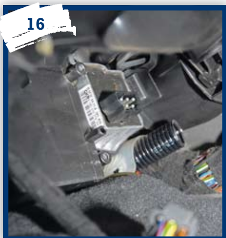
Simply unplug the wiring connector and then ease the retaining clip to one side and slide the resistor out. We found the clip was hard work and the resistor needed a fair bit of wiggling after being in there for nine years.
