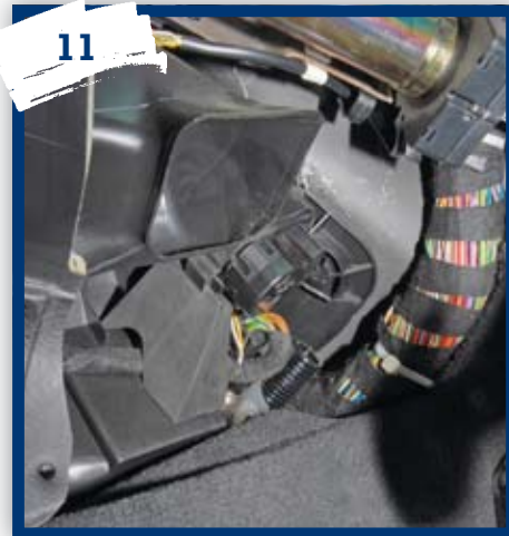
With the trim panel out of the way, you can see the resistor – or at least the general area where it lives. It's partially hidden behind the plastic moulding which houses one of the stepper motors for the air conditioning, and you'll need to remove this before you can slide out the resistor.
