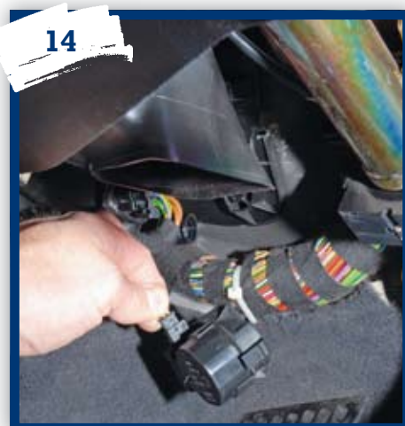
The control linkage can also be unclipped to allow the housing to be removed completely.
