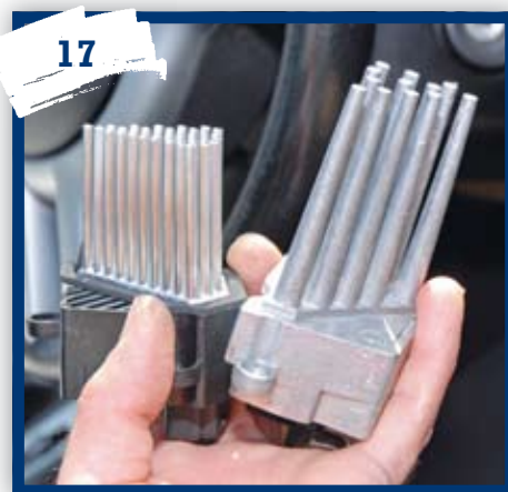
Here you can see the old and new resistors compared, with the new unit from Motormec on the left. Don't worry if they don't look identical as BMW itself went through three designs on the E46 alone. Refitting it is as they say in the best books, the reverse of removal but make sure you seat the new resistor firmly enough for the retaining clip to engage securely.
