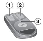
Synchronisation is necessary if the buttons on the remote control unit are pressed more than 256 times outside the range of the receiver. When this limit is reached the receiver on the motorcycle no longer reacts to signals from the remote control unit.
